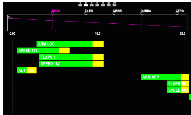
Figure 2: The CHAP-E display with approach profile above, and actions and action windows displayed below
